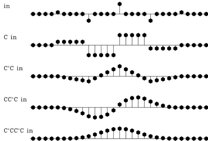
Figure 2: Building the smoothed filter for 3-D antialiasing by successive integration of a five-point wavelet.  $C$  denotes the operator of causal integration,  $C'$  denotes its adjoint (the anticausal integration). The result is equivalent to the convolution of two equal triangle filters.
