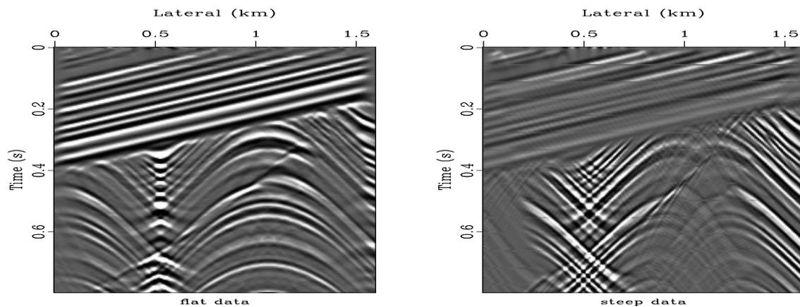
Figure 10: Antialiased modeling. Left corresponds to the flat-dip term. Right corresponds to the steep-dip term.
